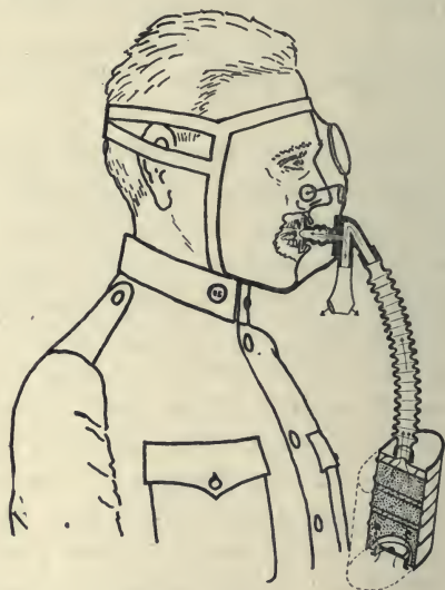
FIG. 53.—Diagrammatic Sketch of Box Respirator Type Mask.
